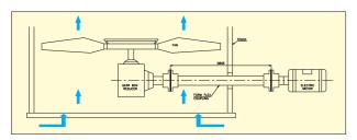
Induced Draft cooling tower drive systems are usually designed with a motor, gearbox, and fan located at the top of the cooling tower.
